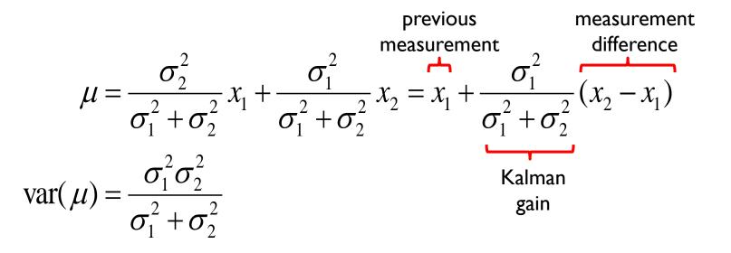
claim: the estimate is a special case of the discrete Kalman filter algorithm
